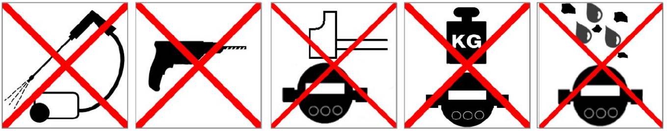
Fig. 8: Prohibited mechanical stress
