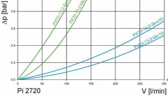
y = differential pressure  $\Delta p$  [bar] x = flow rate V [l/min]
